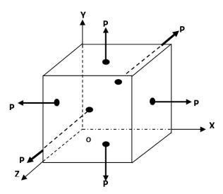
Consider a unit cube as shown in figure. Let the faces of the cube are parallel to the coordinate axes X, Y, Z. Let a Normal Stress P is acting on all the six faces in an outward direction.
