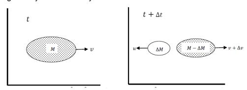
Consider a system of mass M moving with velocity v as shown in figure. After a time  $\Delta t$ , a mass  $\Delta M$  is ejected from the system with velocity u. As a result, mass of the system is reduced to  $(M - \Delta M)$  and its velocity increased to  $(v + \Delta v)$ .
