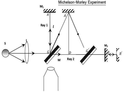
Aim: Aim of Michelson-Morley experiment is to determine the velocity of Earth relative to Ether.
