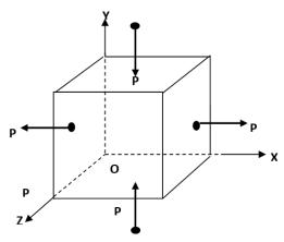
Consider a unit cube as shown in figure. Let an expansive stress P is acting along X axis and a compressive stress P is acting along Y axis on the unit cube.
