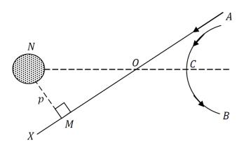
Consider an alpha particle of mass m and charge  $+\ 2e$  moving towards a nucleus of charge  $+\ Ze$  in AX direction. Alpha particle follows a hyperbolic path ACB instead of a straight path AX due to Coulomb's repulsion of the nucleus. p is the perpendicular distance from nucleus N to the initial direction of the alpha particle. This is known as the Impact parameter. Hence Impact parameter can be defined as follows.
