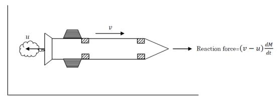
Motion of the rocket is an example of a system of variable mass. When the fuel in the combustion chamber of a rocket is burnt, pressure inside the chamber increases. Hence the hot gases inside the combustion chamber are ejected from the rocket in the form of a gas jet with high velocity in backward direction through a nozzle. Hence mass of the rocket decreases gradually due to the ejected gases and its velocity increases.
