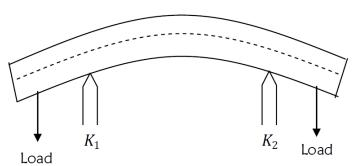
**Non-uniform bending**: If the value of radius R is different for different points of the neutral axis, the bending is called non-uniform bending. The bending of a beam which is symmetrically supported on two knife edges and loaded at the middle is an example for non-uniform bending. Non-uniform bending is shown in figure.
